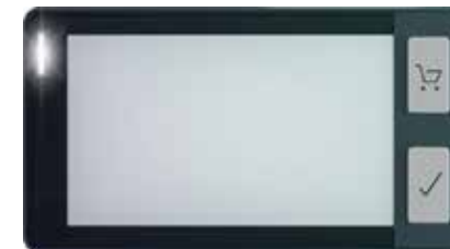
sepioo D2.6 B Size: 80.1 × 40.4 × 13.1 mm Display: 296 x 152 pixel NFC
